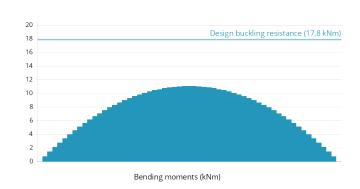
Design bending moment, major axis  $M_{Ed} = 11 \text{ kNm}$ Design resistance for bending  $M_{c,Rd} = 33.8 \text{ kNm}$ Bending utilisation  $M_{Ed} / M_{c,Rd} = 33 \% \text{ OK}$ Design resistance for buckling  $M_{b,Rd} = 17.8 \text{ kNm}$ Buckling utilisation  $M_{Ed} / M_{b,Rd} = 62 \% \text{ OK}$
