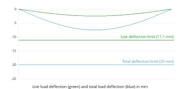
$\begin{array}{lll} \mbox{Variable action deflection limit} & \Delta_{\mbox{\scriptsize Q}} = 11.1 \mbox{ mm} \\ \mbox{Variable action deflection} & \delta_{\mbox{\scriptsize Q}} = 2.5 \mbox{ mm} & \mbox{\scriptsize OK} \\ \mbox{Total deflection limit} & \Delta_{\mbox{\tiny G+Q}} = 20 \mbox{ mm} & \mbox{\scriptsize OK} \\ \mbox{Total deflection} & \delta_{\mbox{\tiny G+Q}} = 7.5 \mbox{ mm} & \mbox{\scriptsize OK} \\ \end{array}$
