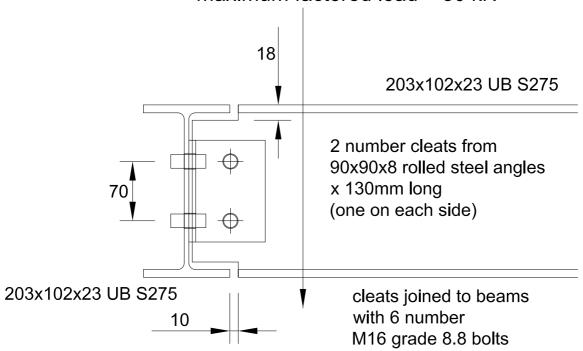
Bearing Capacity of M16 bolt passing through 5.4mm thick S275 steel = 36.8 kN
