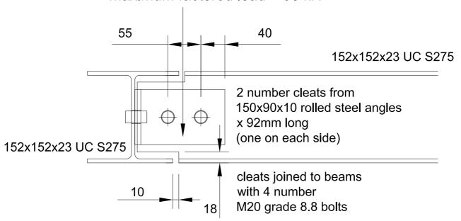
Bearing Capacity of M20 bolt passing through 5.8mm thick S275 steel = 48.8 kN
